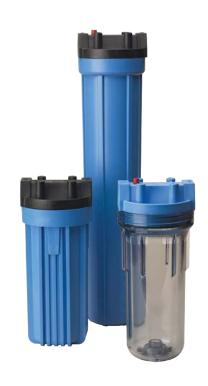
Standard Filter Housings are manufactured of a durable polypropylene or clear FDA-compliant Styrene-Acrylonitrile (SAN). All are equipped with 3/4" NPT inlet and outlet ports. Standard Filter Housings are available in both 10" and 20" lengths and will accommodate a wide range of 2-1/2" to 2-7/8" diameter cartridges. The reinforced polypropylene cap offers an optional pressure relief button on the inlet side to relieve pressure inside the housing when changing filter cartridges.
